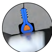
Disc in Closed Position. No line pressure.
